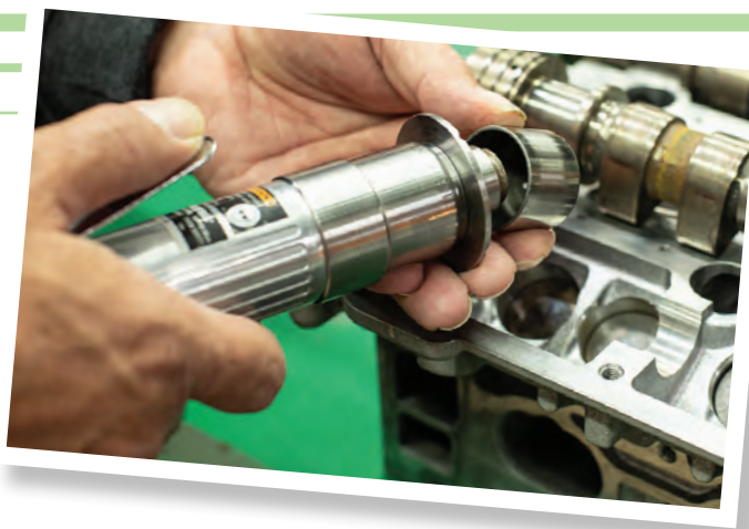
CBN Cutter makes quick work of virtually any bucket lifter
