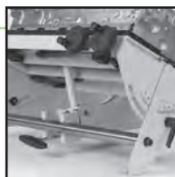
Positive Stops: Adjusts front and rear angles
