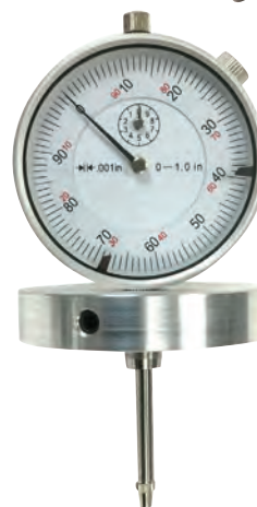
Use the Dial Indicator and Base to measure the valve contact point. Once determined, remove necessary material to set lash.
