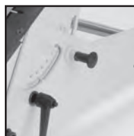
Quick Release Knob: Allows fast positioning to opposite cam bank
